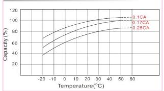
Temperature Effects in Relation to Battery Capacity
